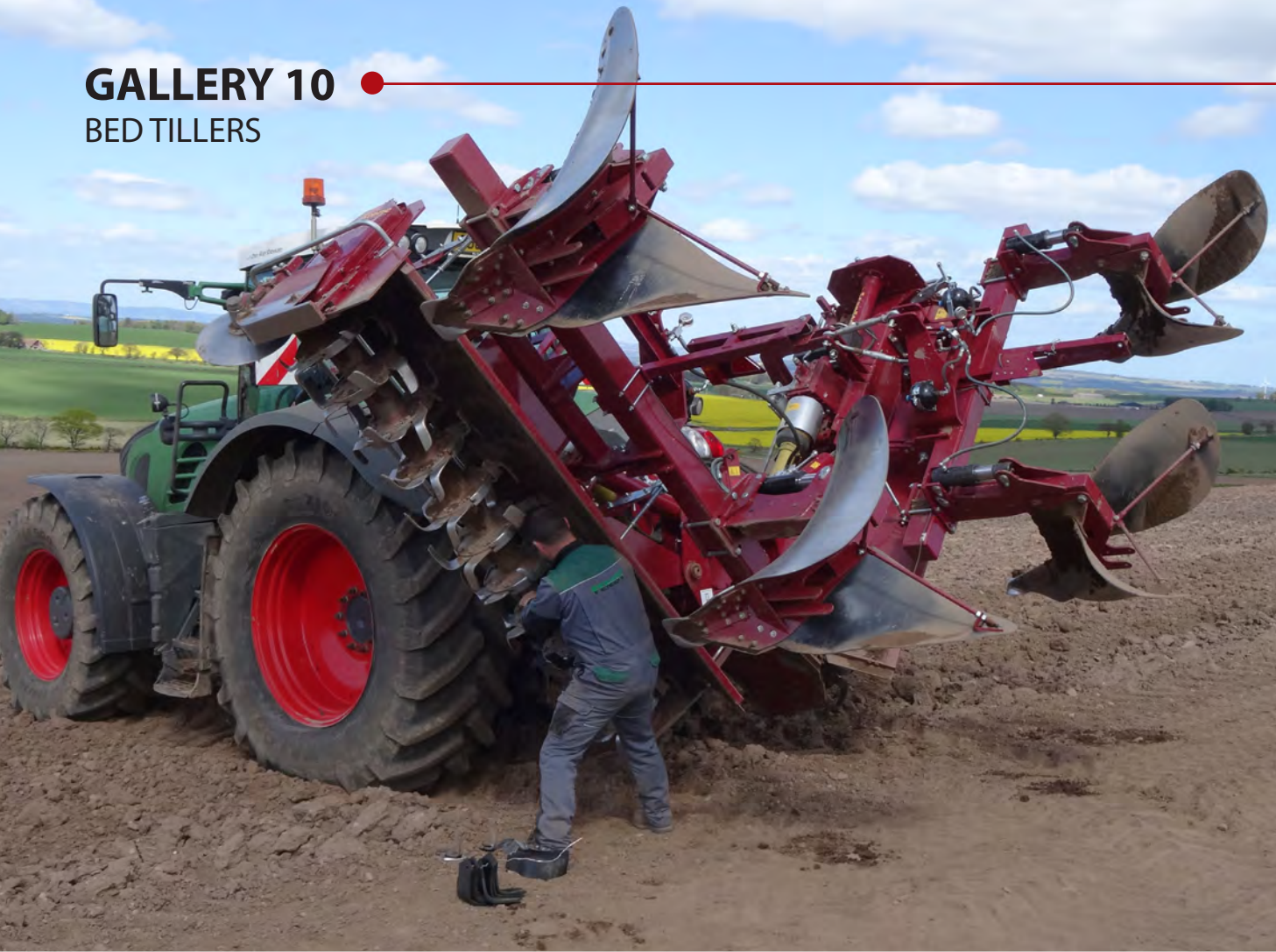
5.4M TRIPLE BED TILLER QUICK CHANGE BLADES
