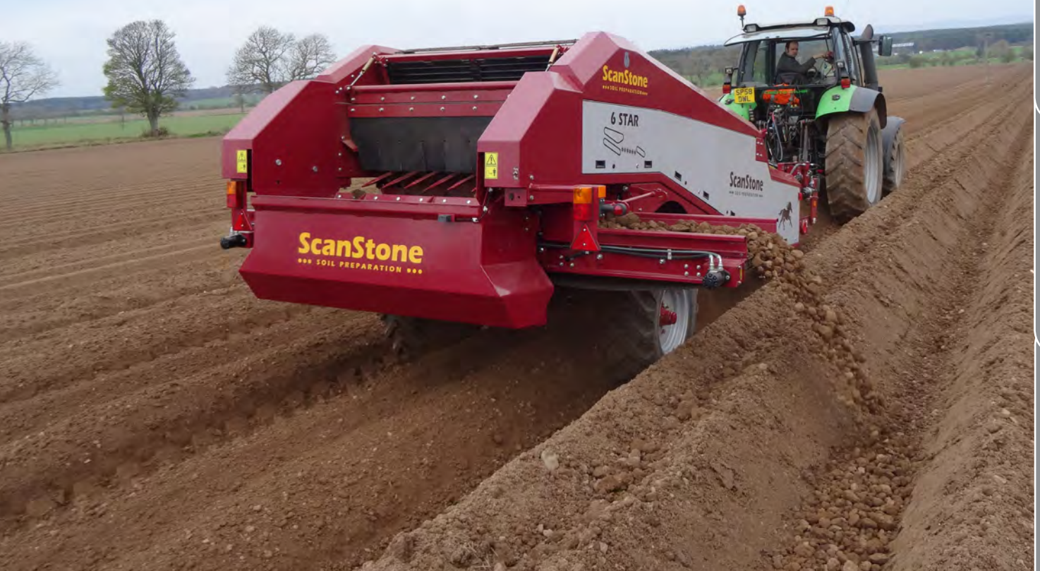
ECOSTAR DESTONER WITH RAKE-TYPE STONE BOX
