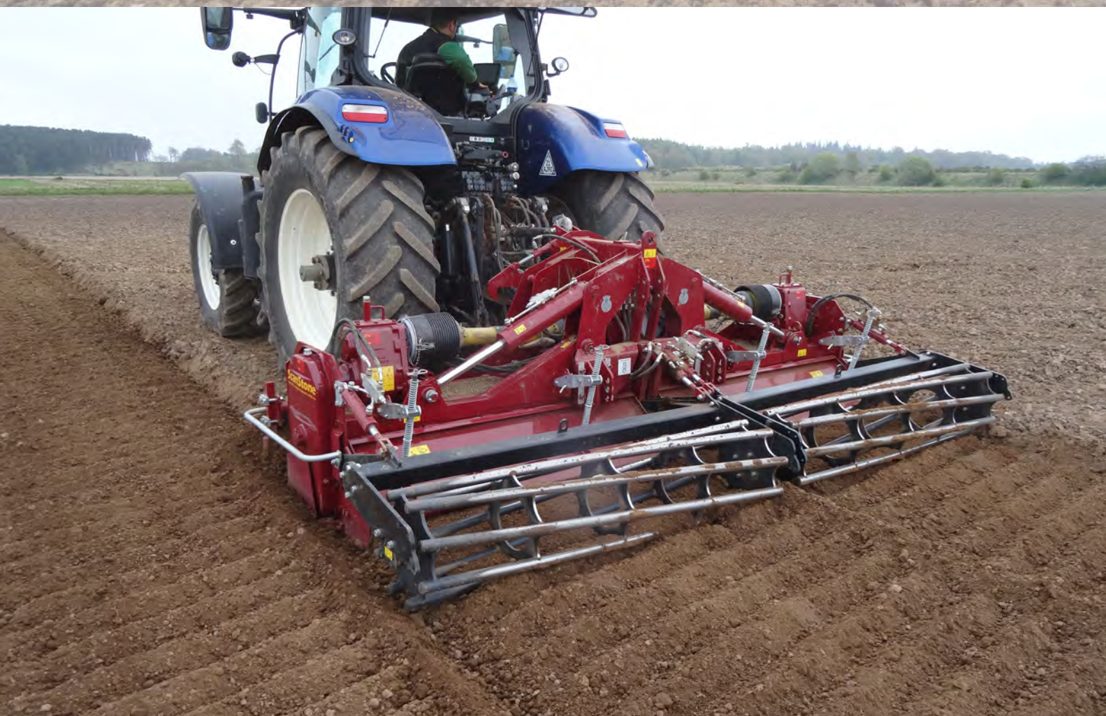
3.6M FOLDING BED TILLER WITH CAGE ROLLERS
