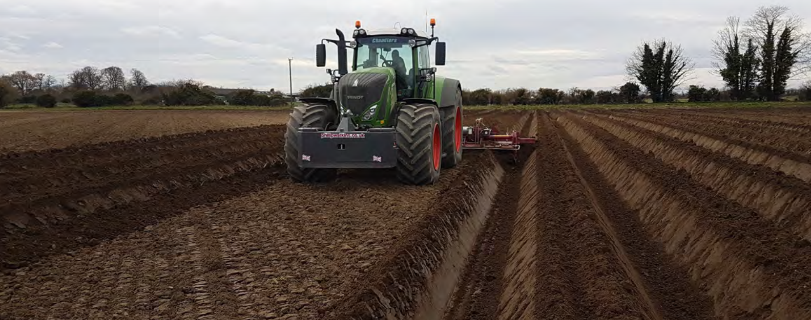
5.4M TRIPLE BED TILLER WITH TWO 2 BODY BED MAKERS
