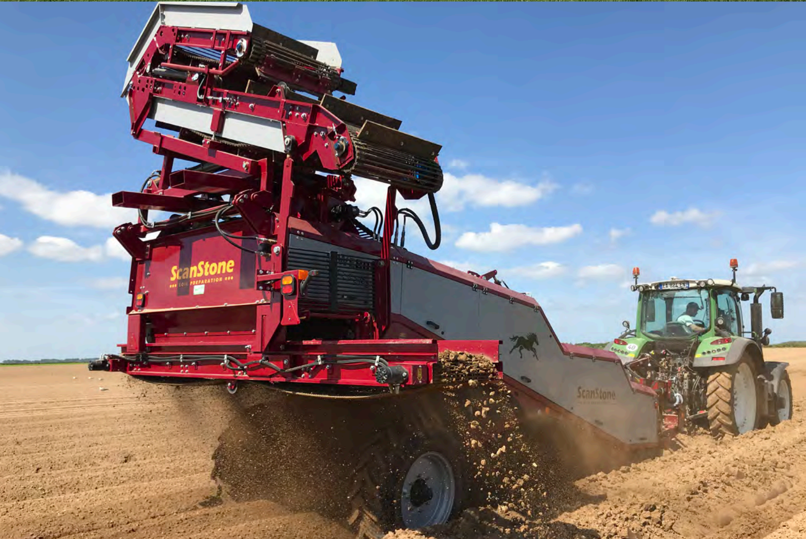
STONE HARVESTING ELEVATOR
