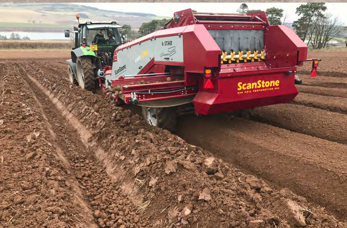
VARI STAR DESTONER WITH STAR TYPE STONE BOX
