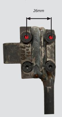
4 Screws Measurable difference between 37mm and 43mm
